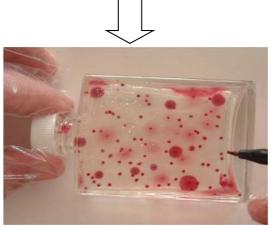
6. To examine test, hold bottle against a light background and count all of the red / purple colonies, marking them off on the bottle with a felt tip pen. Re-incubate and examine if necessary for up to 4 days (see Notes). If numbers are high an estimate can be made by comparison to the chart provided. Record all results and sample information.
