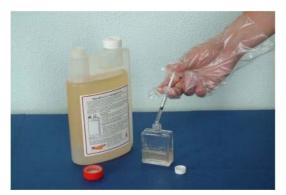
**1.** Break and discard the plastic seal. Remove the bottle cap and place on a clean surface with the inside face upwards. Use the syringe to add 0.25 ml fuel to the MicrobMonitor2 bottle (or 0.01 ml water using the sterile loop). Re-cap and label the bottle.
