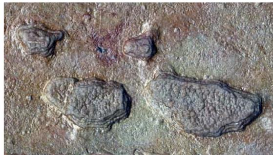
*Pitting Corrosion caused by SRB*
